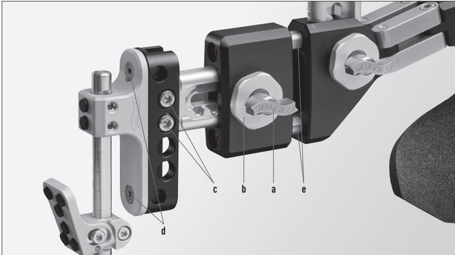
To alter the stock length, undo **the clamping screw (a)**, after which the stock length can be varied by turning **the setting wheel (b)**. Then retighten the setting wheel (b) using the clamping screw (a). If the stock length cannot be extended far enough, a longer stock can be obtained by using longer rods (special accessory). Another way to lengthen the stock is to insert **additional extensions (e)**.
