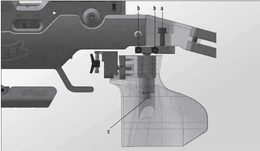
For **longitudinal adjustment and lateral displacement**, undo screw (a) and move the grip to the required longitudinal and lateral position. Lateral displacement is achieved by turning the crosspiece. Then fix this setting using the screw (a).
